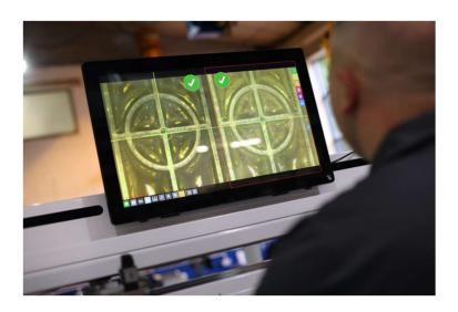
As analogue cameras and monitors have become obsolete and no longer manufactured, we have developed a new digital vision system. HD digital colour cameras display the images on a HD flat screen monitor. The system uses bespoke software running on a fan-less industrial computer with an operating temperature between -20C to +70C at 100% CPU. Benefits include:
